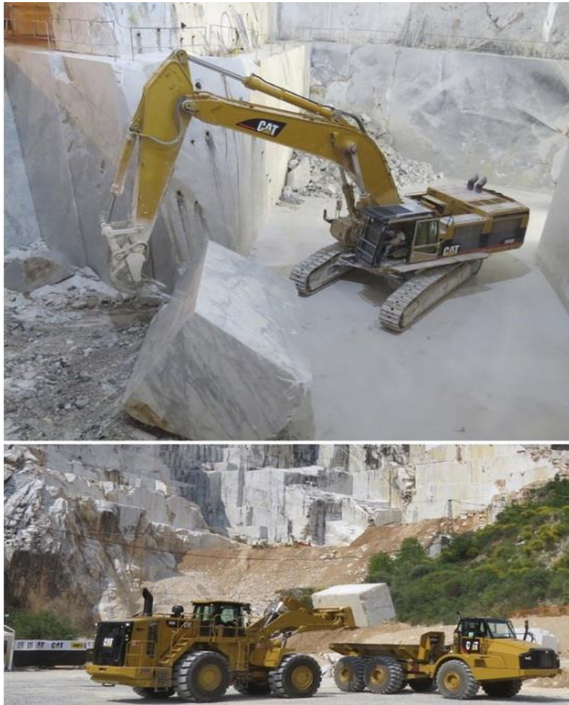
FIGURE 10: MARBLE HANDLING AT QUARRY
