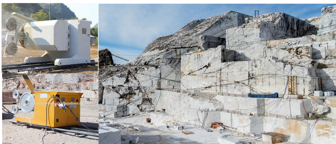
Figure 10: Modern Mechanized Mining in Italy (Diamond Wire Saw)
