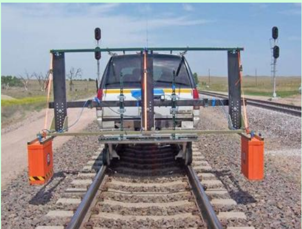
GPR for Railway Track Inspection
